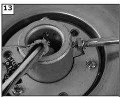
Loosen 2 set screws with lock nuts in yoke till you can not feel them on inside of yoke.
